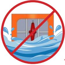
No, the solid outer neoprene sleeve needs to face oncoming water. Under the sleeve are 2 steel plates which slide when adjusting in size and then seal against the frame structure when hit with oncoming water, creating a solid surface. Securing this in the opposite direction will cause these steel plates to spread apart & cause seepage.
